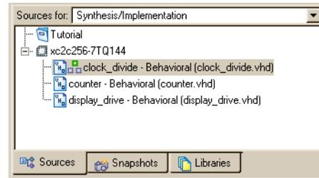
Figure 4-20: Sources in Project Window (Synthesis/Implementation View)
