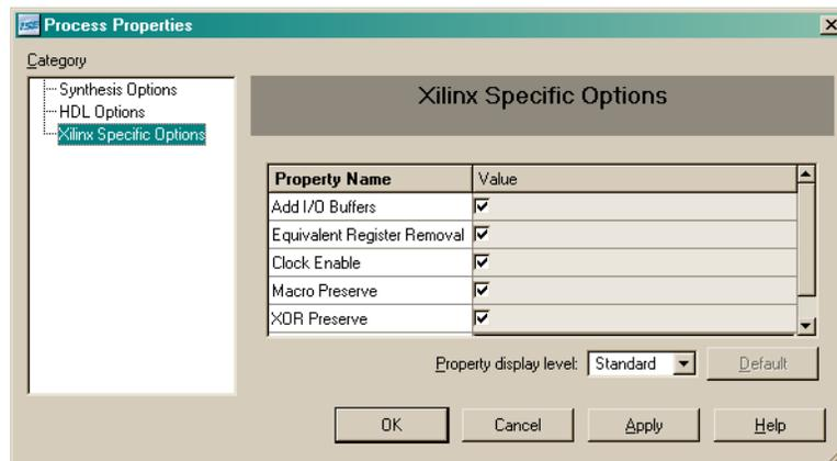
Figure 5-3: Process Properties for Xilinx Specific Options
