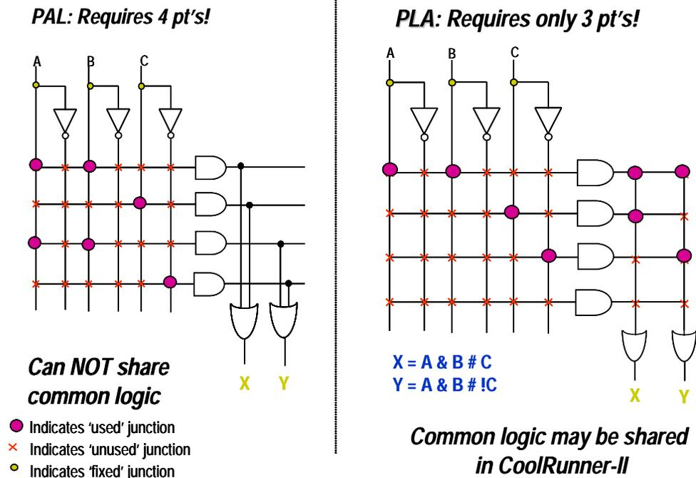
Figure 2-6: Logic Allocation – Typical PAL vs. PLA
