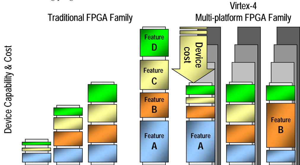
Figure 2-19: Xilinx ASMBL Architecture
