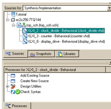
Figure 5-1: Process Window Showing Check Syntax for `clock_divide.vhd`
