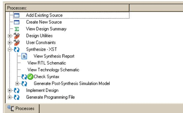
Figure 6-3: Processes Window Showing Check Syntax Success
